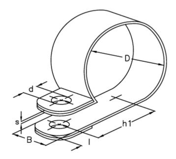
$\begin{array}{ll} d & = 10.5 \\ \text{Diameter D} = 25 \\ \text{h1} & = 27.0 \\ \text{I} & = 10.0 \\ \text{s} & = 1.0 \\ \text{Width B} & = 25 \\ \end{array}$
